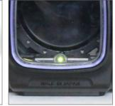
This alarm unit allows you to check waterproofness on land by monitoring the internal pressure by making the inside of the housing negative pressure. When an air leak (change in internal pressure) is detected, an LED lamp warns the user that there is a factor that could cause flooding before entry, thus preventing accidents before they happen. In the unlikely event of water entering the housing underwater, the leak sensor reacts and warns with an LED
