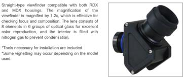
45° viewfinder compatible with MDX housing using an amici prism. Magnification of 1.2x allows for precise composition and focusing. The eyepiece rotates 360° in 90° steps to accommodate a variety of shooting positions, both horizontally and vertically.
