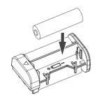
Insert the battery holder straight in the direction of the A.
