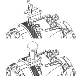
Attach the strobe ball base to the top of the base block using the mounting bolts.
