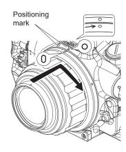
4 Rotate the Port lock lever clockwise until it 'clicks' into position
