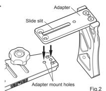
3 Set Washer 1, Washer 2 and Cap Bolt B on the adapter mount holes as shown, then lightly tighten Cap Bolt B using Hex Wrench B (Fig.3)
