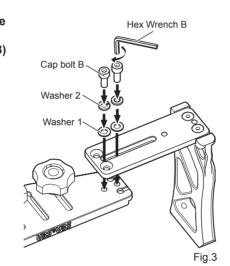
4 Adjust the adapter (grip) position by sliding the adapter into place, and tighten up Cap Bolt B with Hex Wrench B
