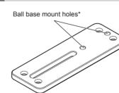
Construction: Corrosion-resistant aluminium alloy (anodized finish) Dimensions (WxHxD): Approx.100×5×35mm /
