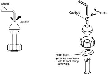
**3** Align the Hook Plate over the rear of the housing accessory shoe, then tighten the Ball Base by rotating the Lock Nut clockwise with the hex wrench.
