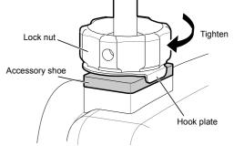
When the Lock Nut cannot be loosened due to salt residue Insert the hex wrench into the Lock nut opening, then turn the hex wrench counter-clockwise.
