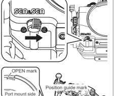
**3.** Align the positioning mark on the front case with the OPEN mark on the port, insert the port into the front case, and then rotate the port in a clockwise direction until it stops
