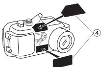
Fit the hole of the Strobe Mask (③) to the Grommet (①), and cut the Strobe Mask in the appropriate shape to attach to the housing.
