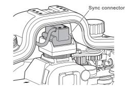
3 When closing the housing, please ensure the connector cord is safely secured inside the housing.
