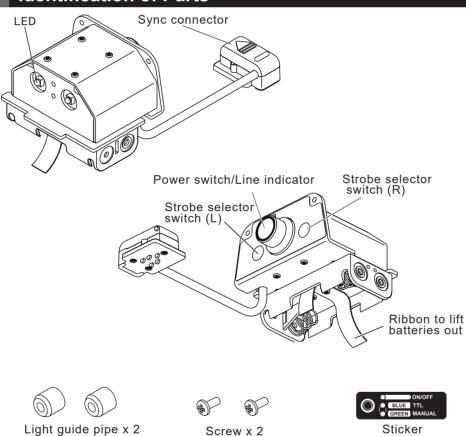
• Use a clean cloth to clean the area for the enclosed supplied sticker and locate a convenient place to stick for easy view.
